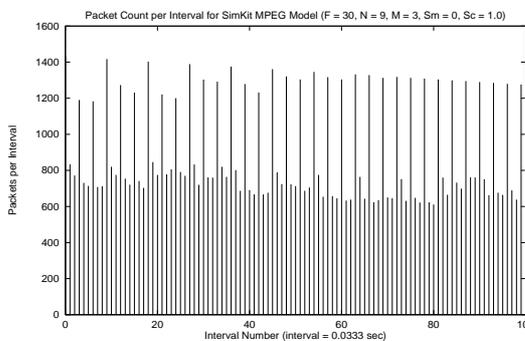
**Figure 6** Packets per time interval for default MPEG GOP at 30 fps, no smoothing
