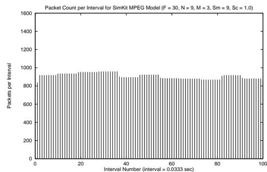
**Figure 7** Packets per time interval for default MPEG GOP at 30 fps, smoothing = 9
