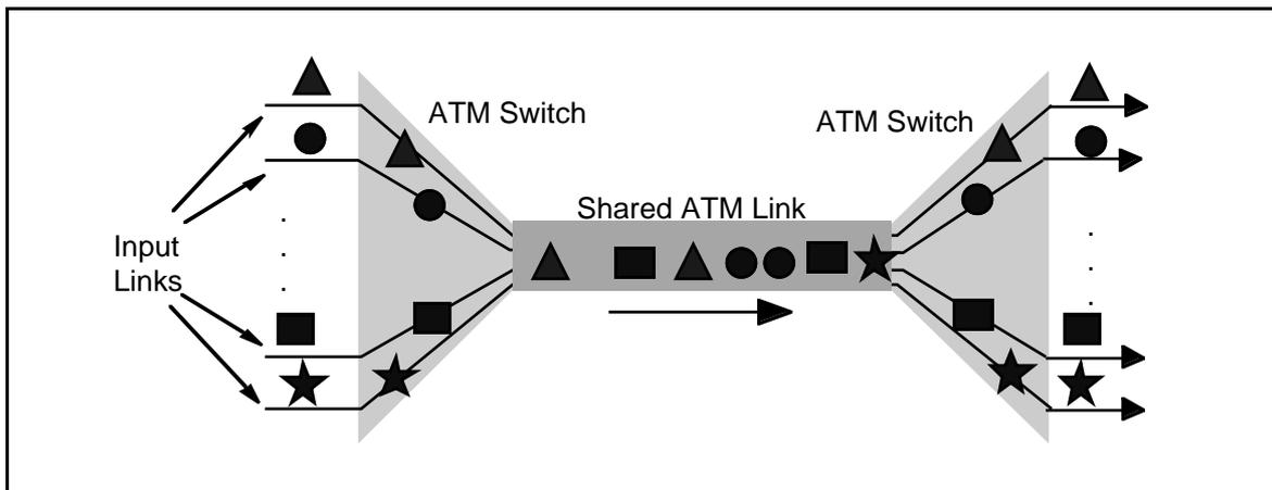
**Figure 2** Statistical Multiplexing on ATM
