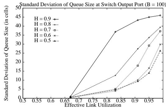
**Figure 10** Standard deviation of queue size at switch output port for ethernet traffic (Chen, et. al., 1995)
