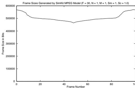
**Figure 5** Frame sizes for MPEG model with only I frames ( $N = 1, M = 1$ )
